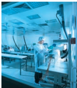
▲ CLASS 100 000 CLEAN ROOM AXON' IS EQUIPPED WITH 2 CLEAN ROOMS
