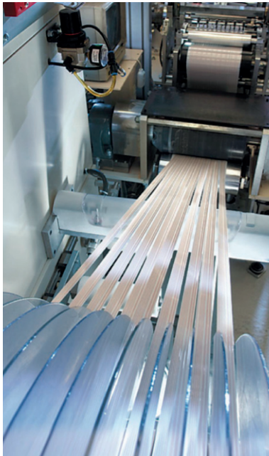
BULK FLAT FLEXIBLE CABLE PRODUCTION
