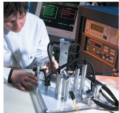
AUTOMATIC CONTINUITY AND INSULATION TESTING
