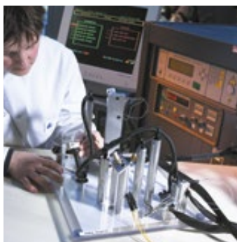
▲ AUTOMATIC CONTINUITY & INSULATION RESISTANCE TEST
