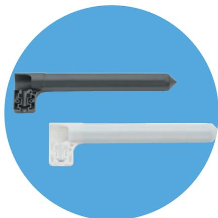
Validation of the final part: molded part on the top and 3D printed prototype on the bottom.
