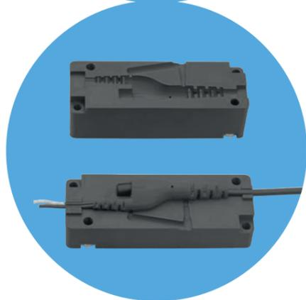
3D printed mold cavities to validate material of the overmolded part.
