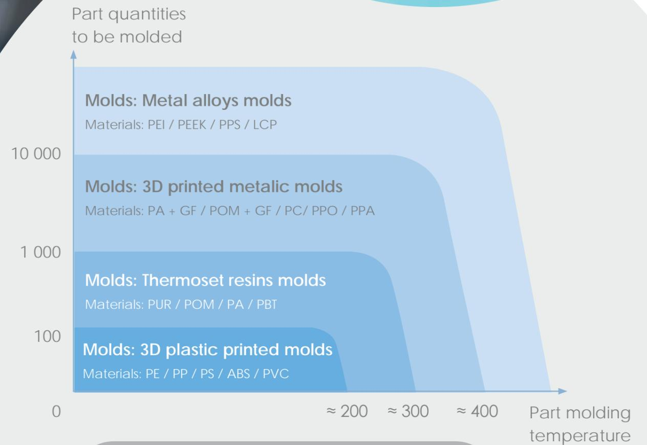
The choice of the mold material depends on the material to be overmolded and the quantity.
